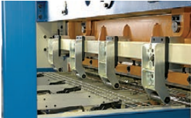
Welding machine mesh feed system (above) and machine's welding portal (below) ...36
