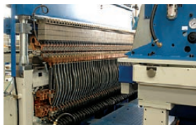
Welding machine mesh feed system (above) and machine's welding portal (below) ...36
