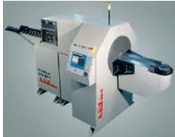
New-concept CNC bending machine...20
