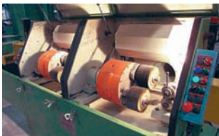
Mechanical descaler with double set of rotating & orbiting wire brushes...36
